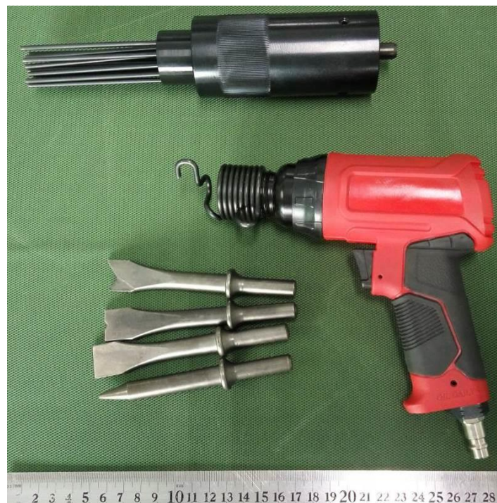
Photo 10: WFH-3140 set (identical with model WFH-3140 except has another accessory as function of Scaling hammer / Needle scaler)
